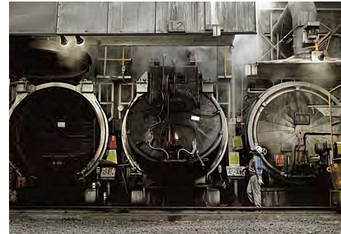
Panels are cured in an autoclave to maximize dimensional stability
